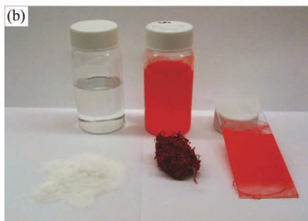
Figure 3 (a) Nanofibers produced with 1 mL of BEH-PPV/PEO solution. (b) Materials used in the production of nanofibers include PEO (white powder), BEH-PPV (red polymer), BEH-PPV in chloroform (container), and resulting nanofibers obtained from solution. [Color figure can be viewed in the online issue, which is available at wileyonlinelibrary.com .]
